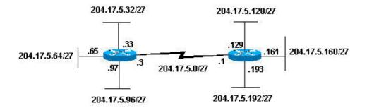
Notice that each of the routers above is attached to four subnetworks, one subnetwork is common to both routers. Also, each router has an IP address for each subnetwork to which it is attached. Each subnetwork could potentially support up to 30 host addresses.
