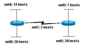
Looking at the above network, you can see that you are required to create five subnets. The largest subnet must support 28 host addresses. Is this possible with a Class C network? and if so, then how?
