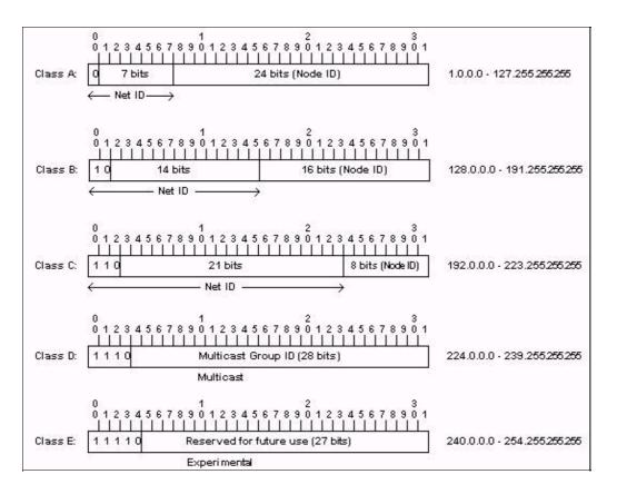
In a Class A address, the first octet is the network portion, so the Class A example above has a major network address of 10. Octets 2, 3, and 4 (the next 24 bits) are for the network manager to divide into subnets and hosts as she sees fit. Class A addresses are used for networks that have more than 65,536 hosts (actually, up to 16,777,216 hosts!).
