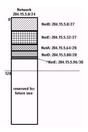
From the above graphic you can see how using VLSM helped save more than half of the address space.
